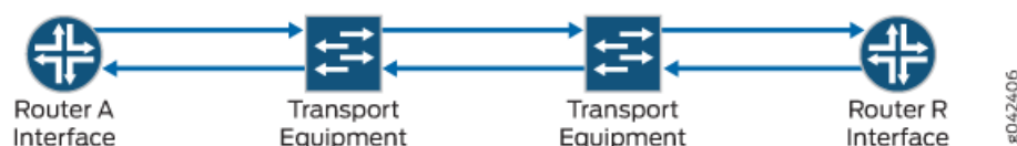
Figure 6: Two Router Interfaces Connected Through Transport Equipment
