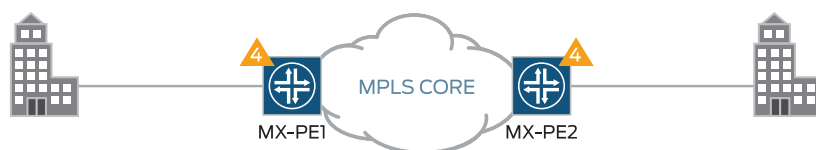
Figure 26: VPWS Service Configured Between Two MX Series Routers
