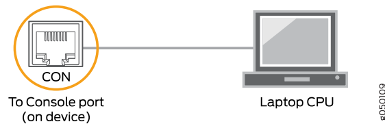
Figure 39: Connecting the QFX Series Directly to a Management Console
