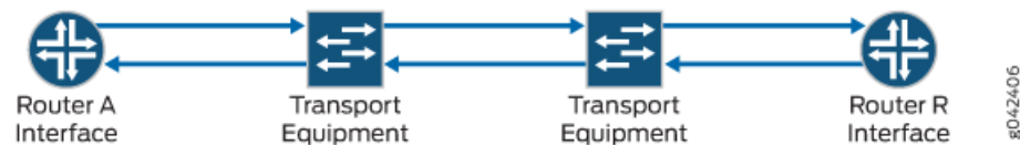
Figure 6: Two Router Interfaces Connected Through Transport Equipment
