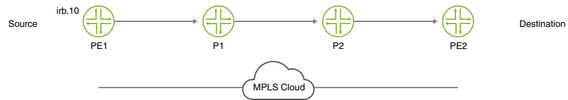
Figure 38: Sampling on an IRB Interface Routing Traffic to a Tunnelled Core
