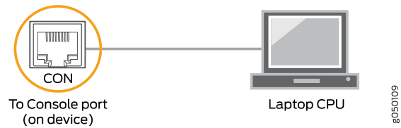
Figure 66: Connecting the QFX Series Directly to a Management Console
