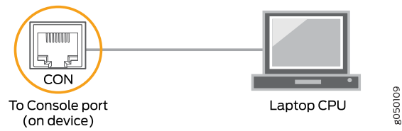
Figure 63: Connecting the QFX Series Directly to a Management Console
