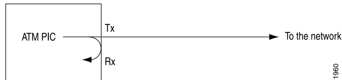
Figure 5: Local Loopback
