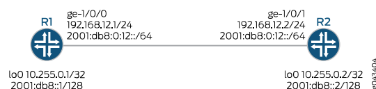
Figure 87: Example LDP Native IPv6 Support
