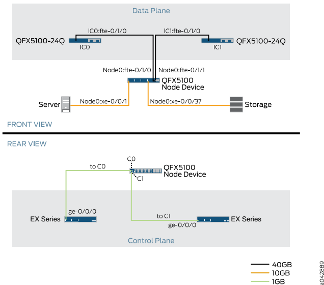
Figure 11: QFX5100 Data Plane and Control Plane Connections
