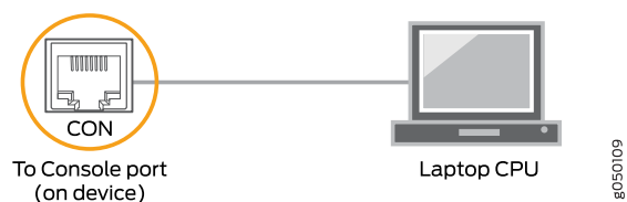
Figure 55: Connecting the QFX Series Directly to a Management Console
