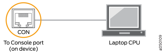
Figure 76: Connecting the QFX Series Directly to a Management Console
