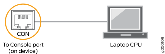
Figure 68: Connecting the QFX Series Directly to a Management Console
