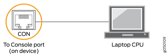
Figure 55: Connecting the QFX Series Directly to a Management Console
