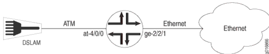
Figure 21: ATM-to-Ethernet Interworking
