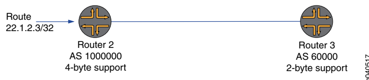
Figure 22: 4-Byte Capable Router Having a Peer Relationship with a 2-Byte Capable Router Using a 4-Byte AS Number
