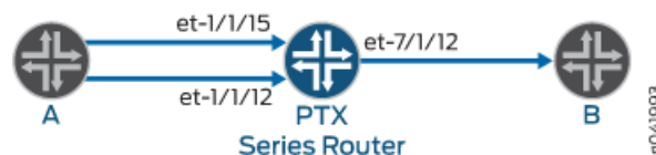
Figure 58: Topology for Configuring Strict-Priority Scheduling on a PTX Series Router
