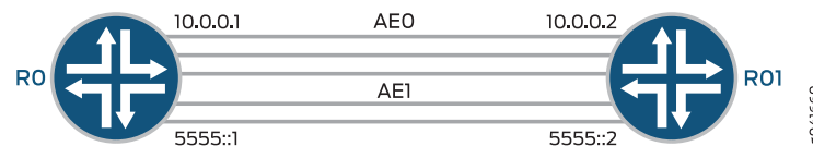
Figure 5: Configuring an Independent Micro BFD Session for LAG
