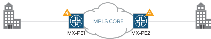
Figure 53: VPWS Service Configured Between Two MX Series Routers
