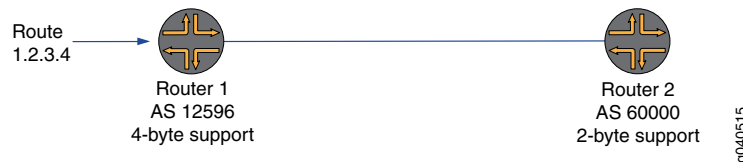
Figure 21: 4-Byte Capable Router Having a Peer Relationship with a 2-Byte Capable Router Using a 2-Byte AS Number
