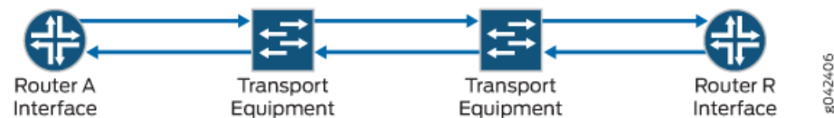
Figure 6: Two Router Interfaces Connected Through Transport Equipment
