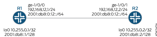
Figure 87: Example LDP Native IPv6 Support
