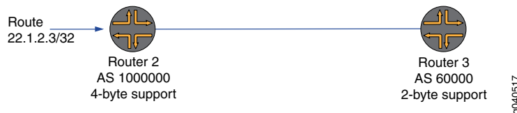
Figure 21: 4-Byte Capable Router Having a Peer Relationship with a 2-Byte Capable Router Using a 4-Byte AS Number
