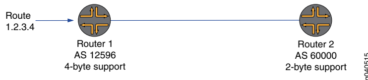
Figure 20: 4-Byte Capable Router Having a Peer Relationship with a 2-Byte Capable Router Using a 2-Byte AS Number
