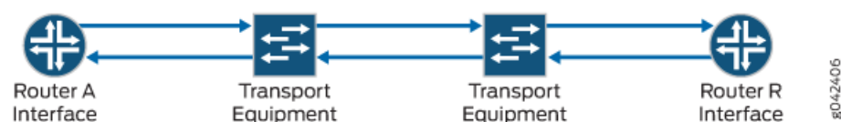
Figure 6: Two Router Interfaces Connected Through Transport Equipment
