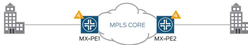
Figure 49: VPWS Service Configured Between Two MX Series Routers
