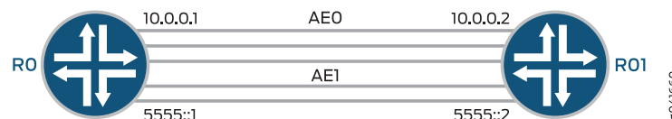
Figure 10: Configuring an Independent Micro BFD Session for LAG
