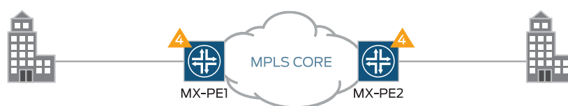
Figure 50: VPWS Service Configured Between Two MX Series Routers
