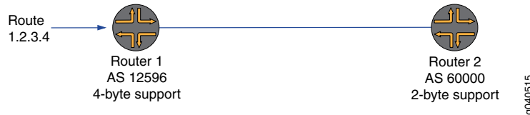
Figure 20: 4-Byte Capable Router Having a Peer Relationship with a 2-Byte Capable Router Using a 2-Byte AS Number
