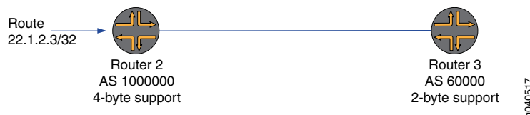
Figure 21: 4-Byte Capable Router Having a Peer Relationship with a 2-Byte Capable Router Using a 4-Byte AS Number
