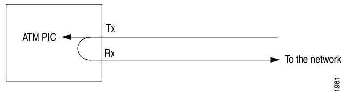
Figure 6: Loop from the Router to the Network
