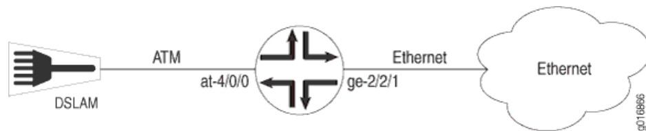
Figure 6: ATM-to-Ethernet Interworking
