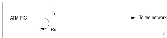
Figure 9: Local Loopback
