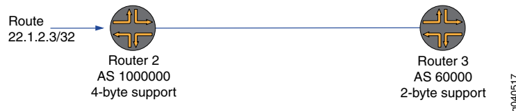
Figure 2: 4-Byte Capable Router Having a Peer Relationship With a 2-Byte Capable Router Using a 4-Byte AS Number
