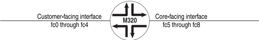
Figure 11: Customer-Facing and Core-Facing Forwarding Classes
