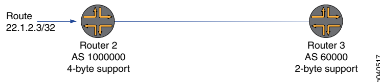
Figure 2: 4-Byte Capable Router Having a Peer Relationship With a 2-Byte Capable Router Using a 4-Byte AS Number
