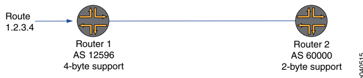
Figure 1: 4-Byte Capable Router Having a Peer Relationship With a 2-Byte Capable Router Using a 2-Byte AS Number
