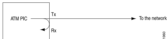
Figure 9: Local Loopback
