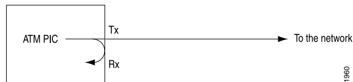
Figure 9: Local Loopback
