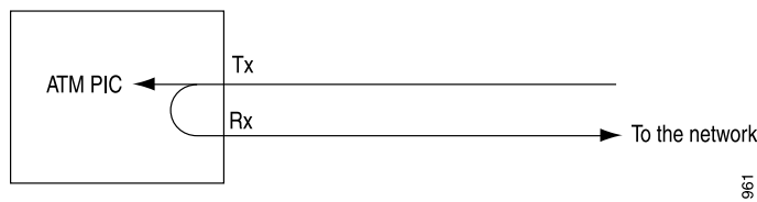
Figure 10: Loop from the Router to the Network
