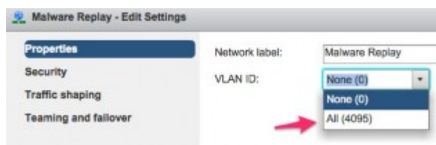
Figure 2: vSwitch VLAN Troubleshooting Config in port-groups
