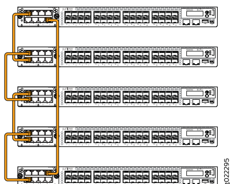
Figure 40: EX4550 Switches Mounted on a Single Rack and Connected in a Ring Topology Using 8-port 10GBASE-T Expansion Module and Using Short and Long Cables: Example 1
