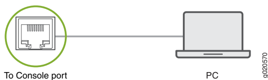
Figure 41: Connect a Device Directly to a Management Console
