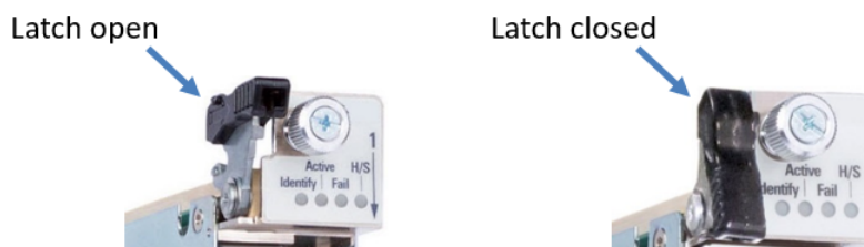
Figure 33: Top Latch - UFM4
