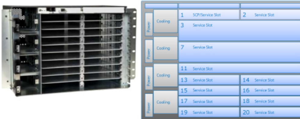
Figure 2-16 BTI 7200 configured to accommodate a packetVX 12/2 module
