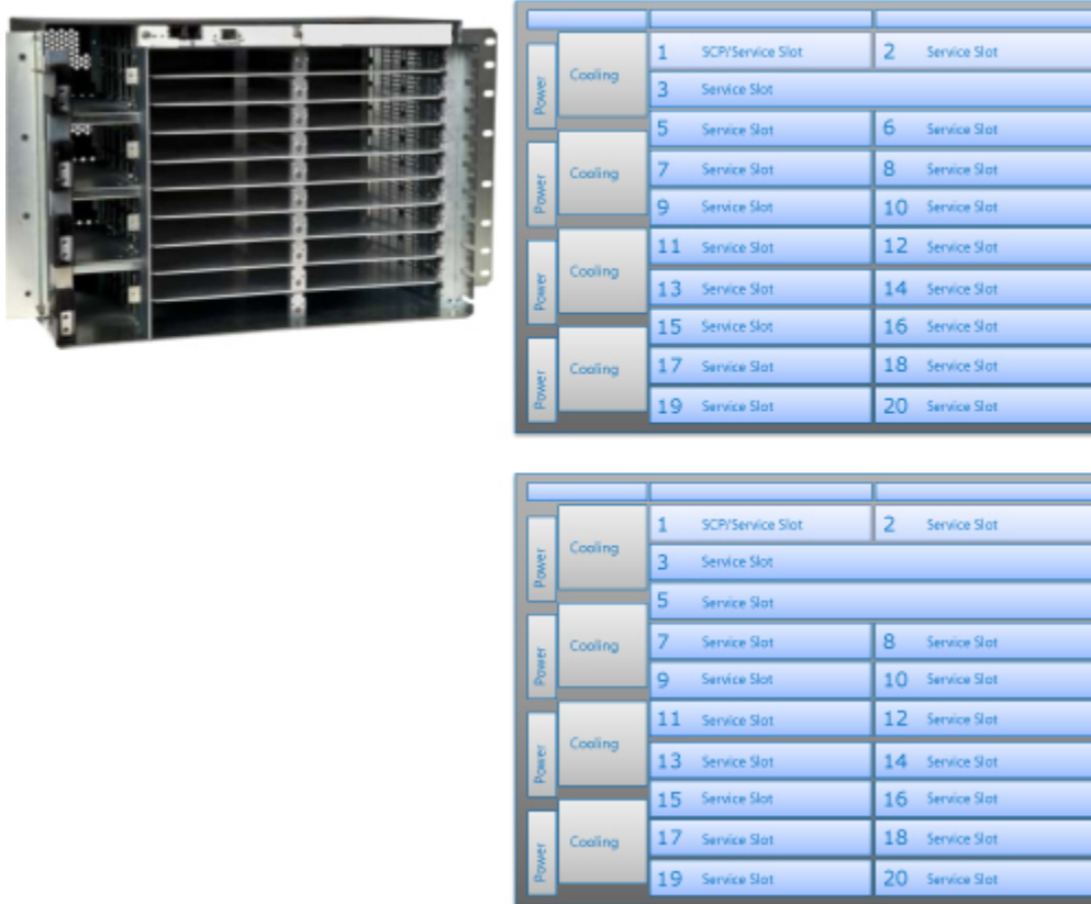
Figure 2-16 BTI 7200 configured to accommodate a packetVX 12/2 module
