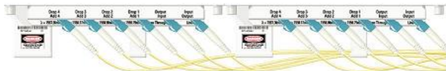
Top View of Optical Fiber Management for Cables with Long Boots
