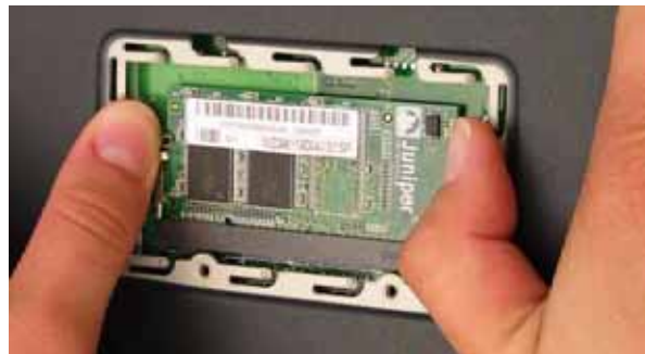
Figure 12: Unlocking the Memory Module
