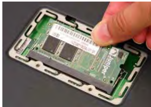
Figure 13: Removing Module Slots
