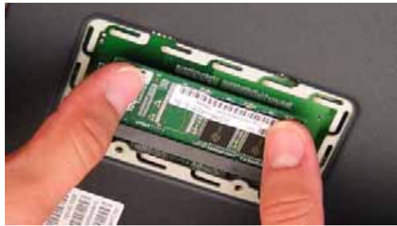
Figure 14: Inserting the Memory Module
