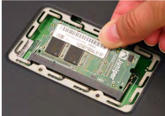
Figure 15: Removing Module Slots
