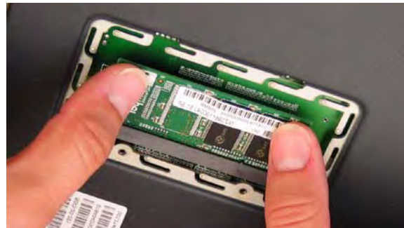
Figure 16: Inserting the Memory Module
