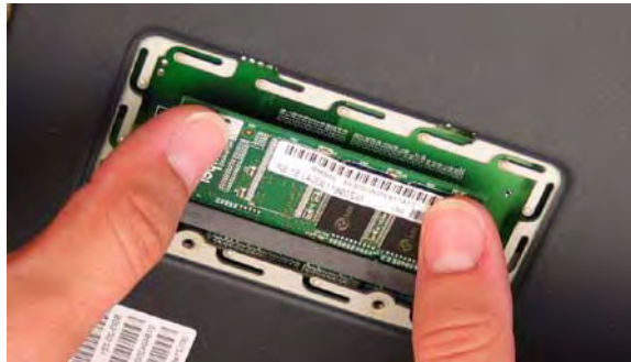
Figure 17: Inserting the Memory Module
