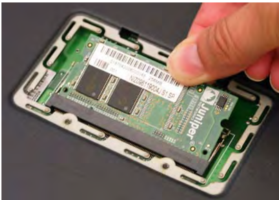
Figure 16: Removing Module Slots
