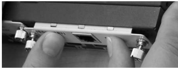
Figure 13: Installing a Mini-PIM
