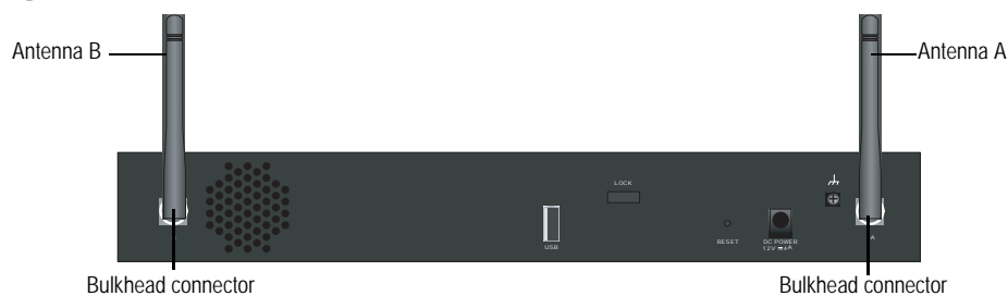
Figure 9: SSG 20-WLAN Antennae Location
