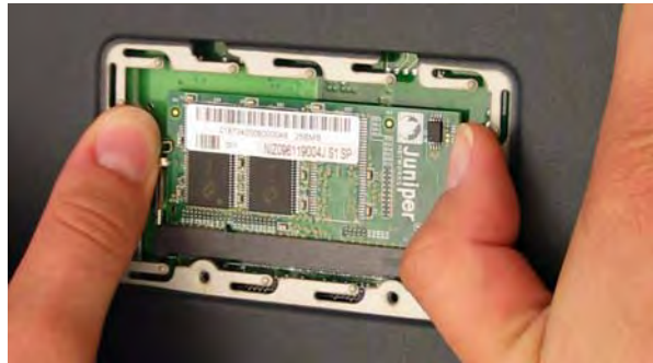
Figure 15: Unlocking the Memory Module
