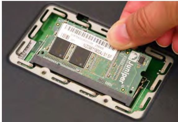
Figure 20: Removing Module Slots
