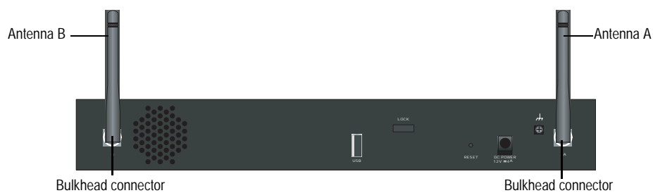
Figure 12: SSG 20-WLAN Antennae Location
