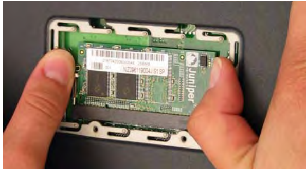
Figure 19: Unlocking the Memory Module
