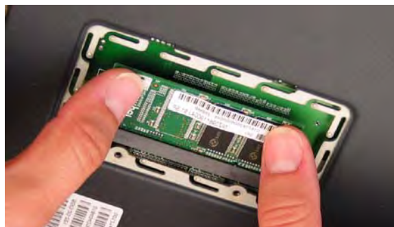
Figure 21: Inserting the Memory Module
