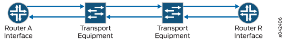
Figure 6: Two Router Interfaces Connected Through Transport Equipment
