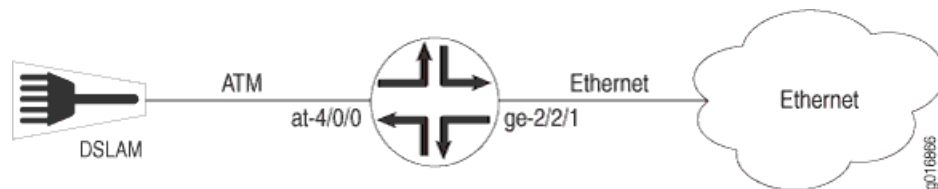
Figure 21: ATM-to-Ethernet Interworking
