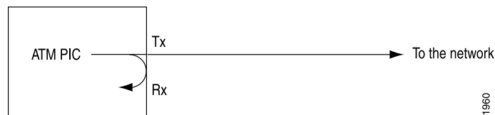
Figure 5: Local Loopback
