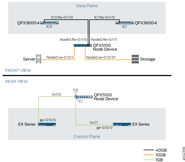
Figure 91: QFX5100 Node Device Data Plane Connects for QFX3000-M QFabric System
