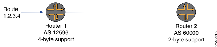
Figure 7: 4-Byte Capable Router Having a Peer Relationship With a 2-Byte Capable Router Using a 2-Byte AS Number
