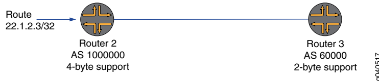
Figure 8: 4-Byte Capable Router Having a Peer Relationship With a 2-Byte Capable Router Using a 4-Byte AS Number
