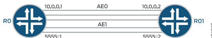
Figure 4: Configuring Independent Micro BFD Session for LAG
