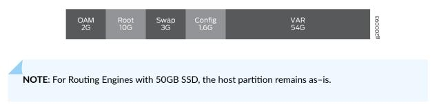
Figure 8 on page 352 and Figure 9 on page 352 illustrates the host partition table and the storage allocation of the guest VM for the MX2010 and MX2020 routers respectively.
