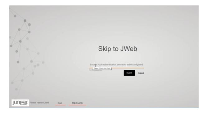
**NOTE**: For SRX1500 devices, the **Skip to JWeb** option is not supported. To access J-Web, the ZTP client configuration must be deleted during the initial setup of SRX1500 through CLI.
